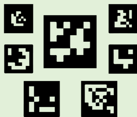
Markers Made Up From Black And White Grids Can Be Detected By Computer Vision
