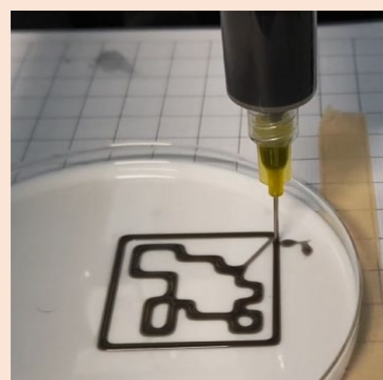
Printing Of Marker Using PDMS Ink
